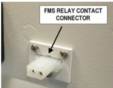
Figure 8. FMS Relay Contact Connector on Rear Panel
